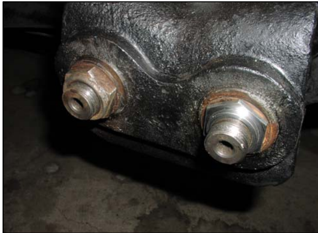
Photo 8 Original nut on left, special machined shoulder nut on the right
