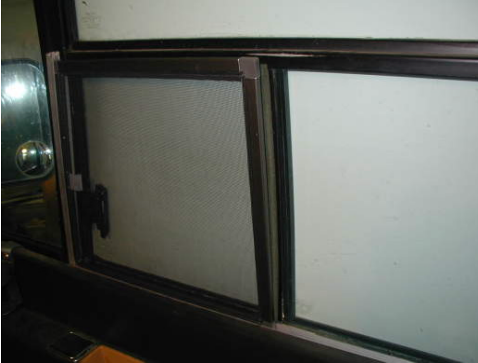
Picture 3: Place the screen in the bottom rail of the screen frame and up against the front rail.
