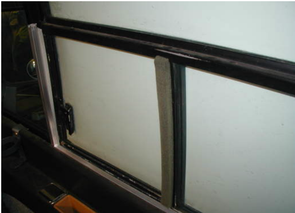
Picture 2: Pull armrest towards you so that you can tuck the bottom rail of the screen
